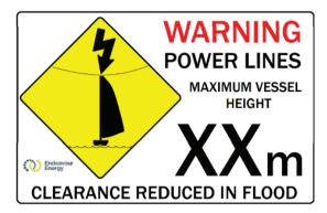
Where there is a risk of contact, prominent warning signage is installed to minimise the possibility of masts contacting overhead powerlines.
