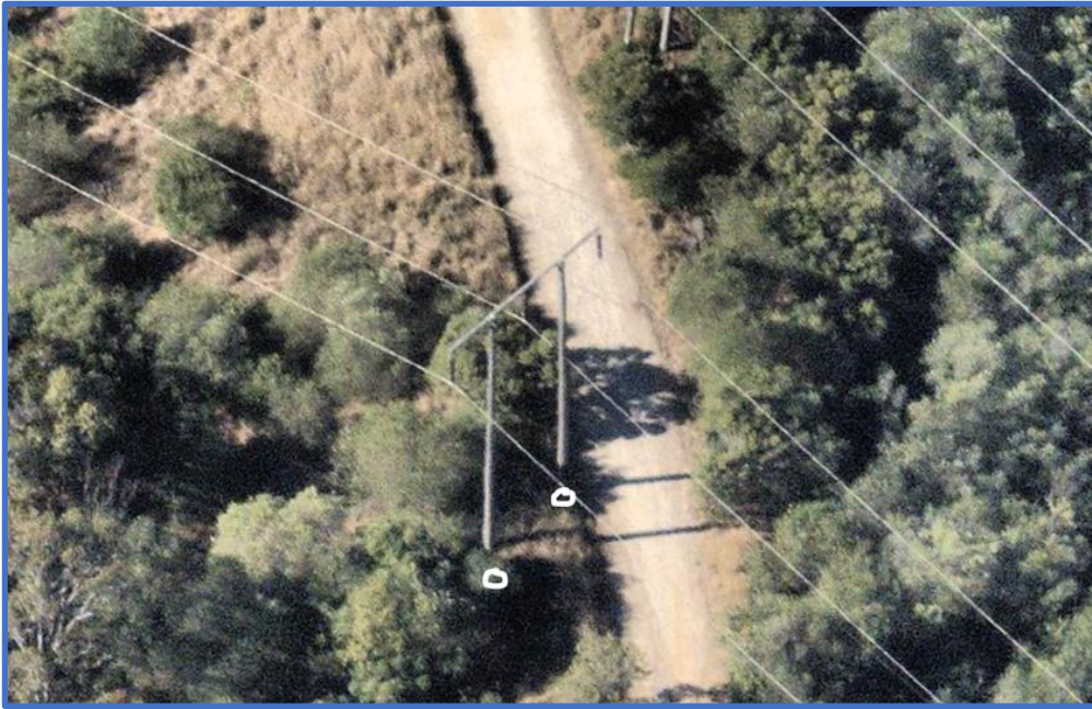
Figure 36: Satellite image showing Pole 15 with markup indicating approximate proposed position of replacement poles
