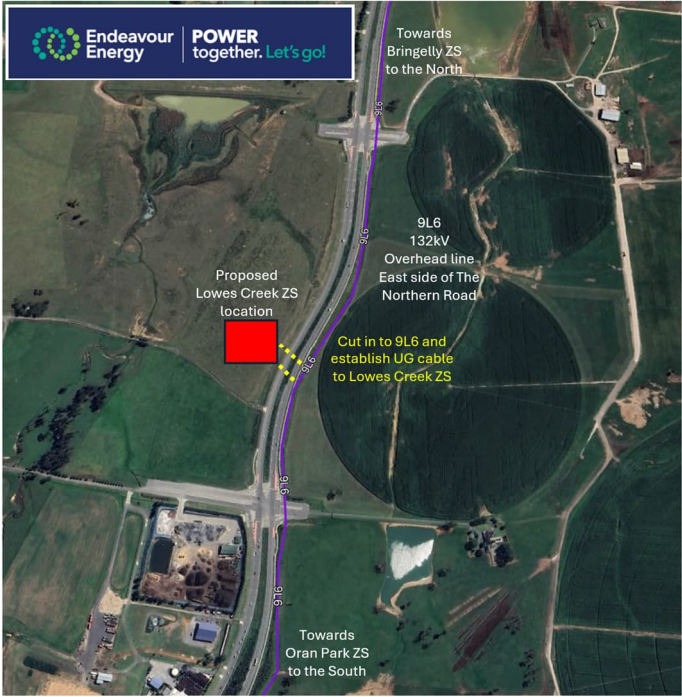
Figure 11 – Proposed 132kV supply to the Lowes Creek zone substation
